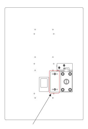
New holes may have to be drilled in this area depending on the location of the postal lock assembly
